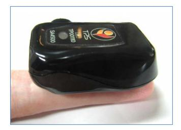
3. Secure the TPS sensor to your finger by wrapping the fabric strap around your finger and back over the TPS sensor. Use the appropriately positioned hole to attach the strap to the central hook on the side of the sensor.
