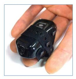
When properly fastened, the fabric strap will cover the TPS sensor logo, but the indicator light will be visible when the sensor is on.
