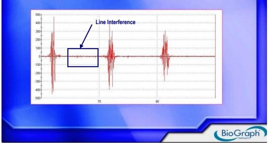
Fig. 3. Raw EMG signal with line interference
