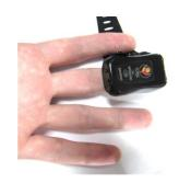
3. The sensor should be placed at the end of your finger. The two metal plates on the underside of the sensor rest against your skin as shown.
