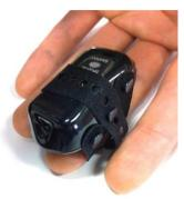
We advice to apply the sensor at least 2-3 minutes before recording a session. This is due to the temperature sensing component, which requires that time to "warm up" to the client's current temperature.
