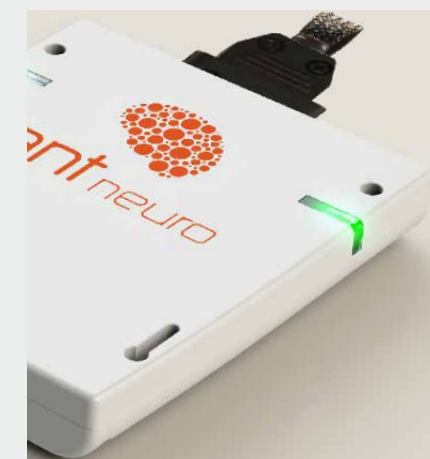
The lights located on the upper left and right side indicate when data is being acquired
